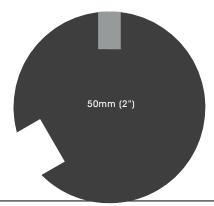
Diameter ø50mm (2") Recommended maximum distance between brackets 2400mm (96")
