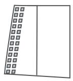
The first hook always goes into the third pocket from the leading edge and then hooks are inserted as required according to the relevant pocket factor (see below).
