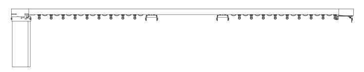
Supplied with 2x Ripplefold Butt Arm. 1x Motor Ripple Sleeve. 1x Return Ripple Plate.
